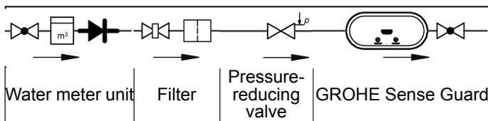
Leakage protection is provided as soon as GROHE Sense Guard is connected to the power supply.
